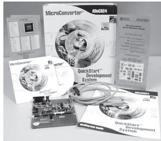
Figure 65. Components of the QuickStart Development System
